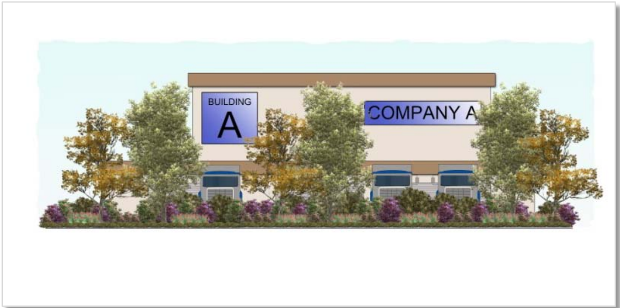
FIGURE 4-7 CONCEPT TO SCREEN DOCKS, ROLL-UP DOORS, AND PARKING AREAS WITH BUILDING-MOUNTED SIGNS
