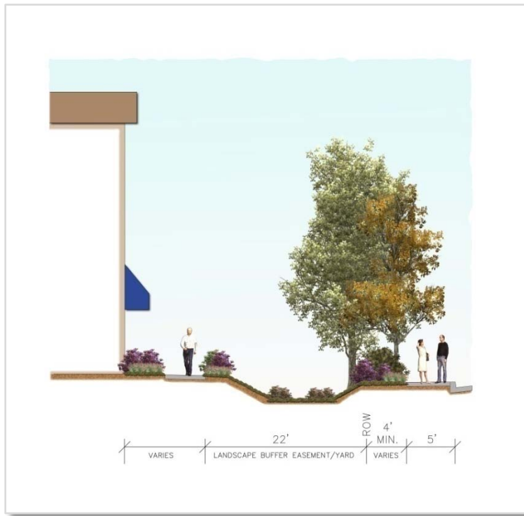
FIGURE 4-3 LANDSCAPE BUFFER EASEMENT ADJACENT TO PRIVATE ENTRY/SIDEWALK
