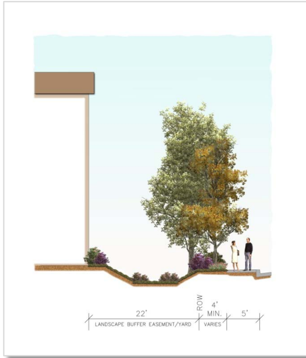
FIGURE 4-2 LANDSCAPE BUFFER EASEMENT ADJACENT TO BUILDING
