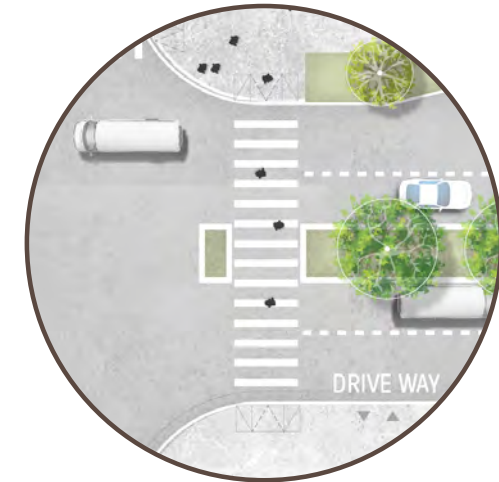
PEDESTRIAN PROTECTION ISLAND
