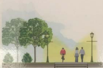
Desired width of two-way bike path: 12 feet
