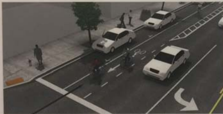
Desired width of buffer: 3 feet Desired minimum width of bike lane next to on street parking: 5 feet
